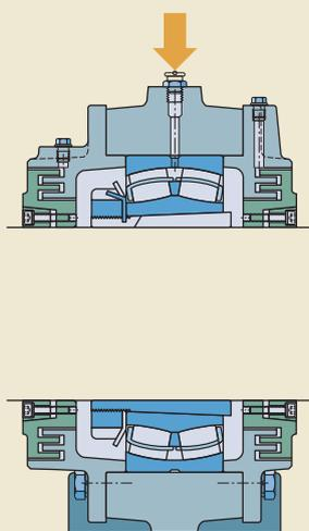
Grease fitting in SBD housing
